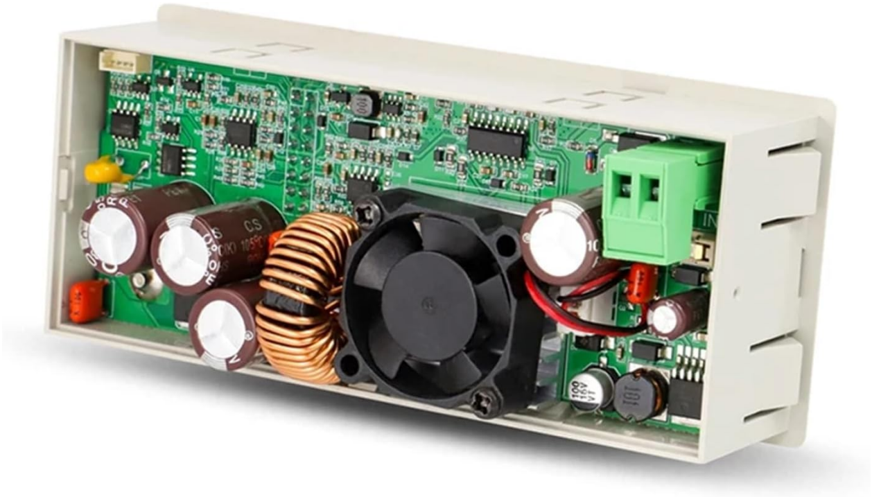
Image 4: Internal components of the XY6008-W module, including the cooling fan and main circuit board.
