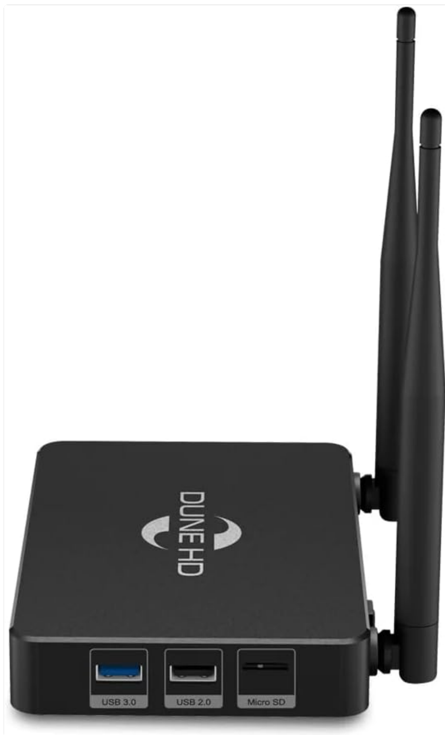
Image: Side view of the Dune HD Pro Vision 4K Media Player, showing the USB 3.0, USB 2.0, and MicroSD card slots.
