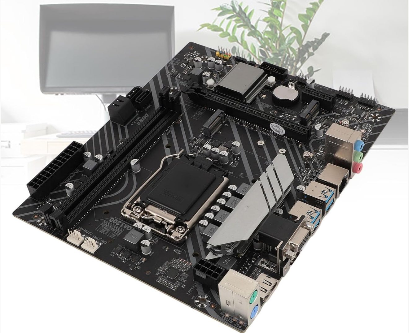
Figure 4.2: The rear I/O panel of the motherboard, featuring various connectivity options including USB, video outputs, and network ports.
