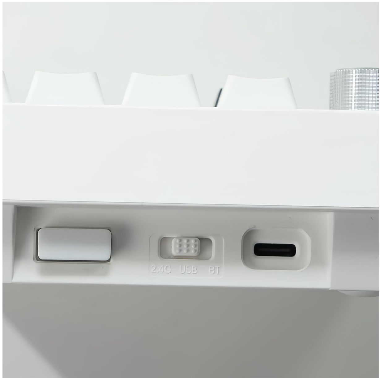
Rear view showing the USB-C port and the switch for 2.4G wireless, USB wired, and Bluetooth modes.
