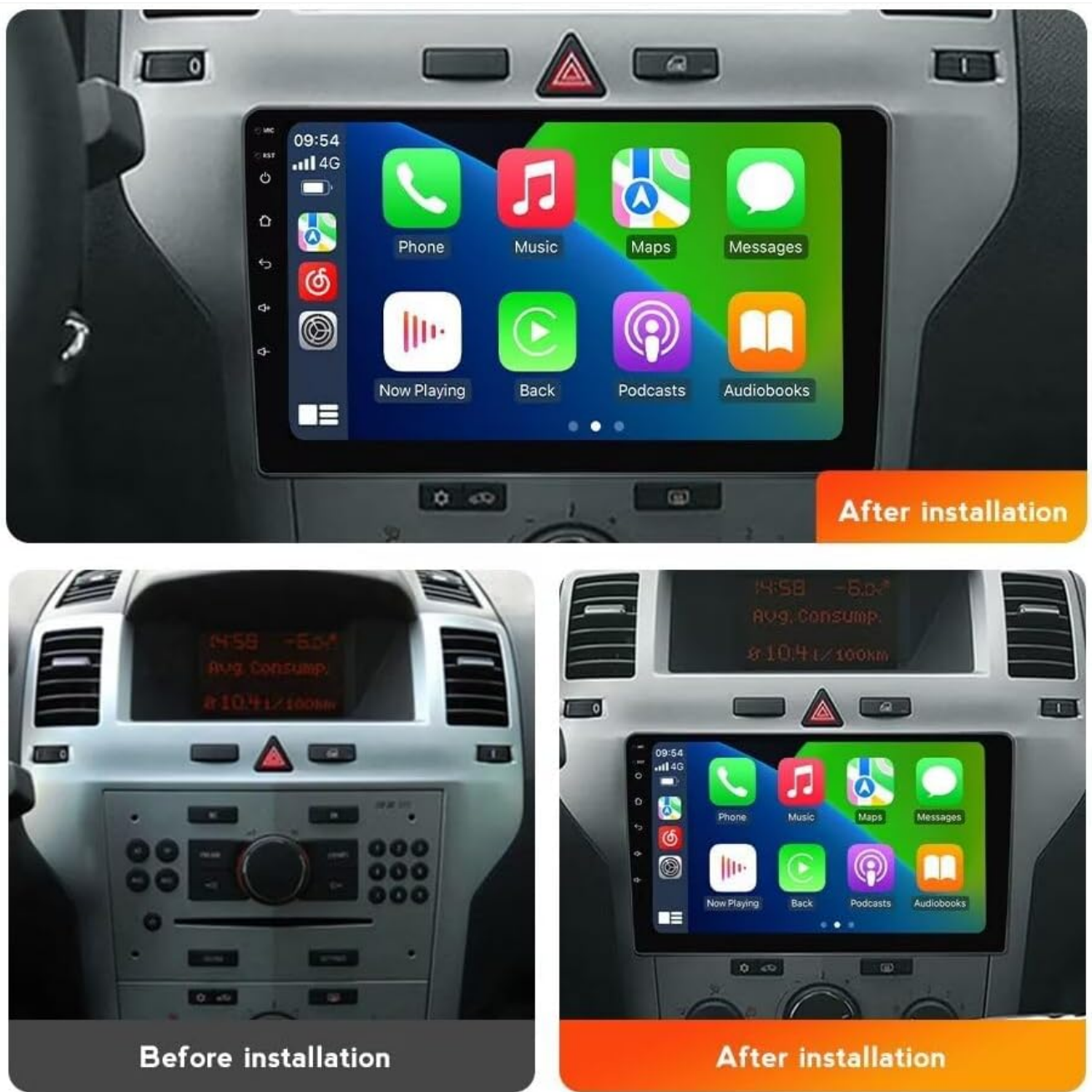
Figure 3.1: Visual comparison of the Opel Astra H dashboard before and after the RONGJI Android Car Radio installation.
