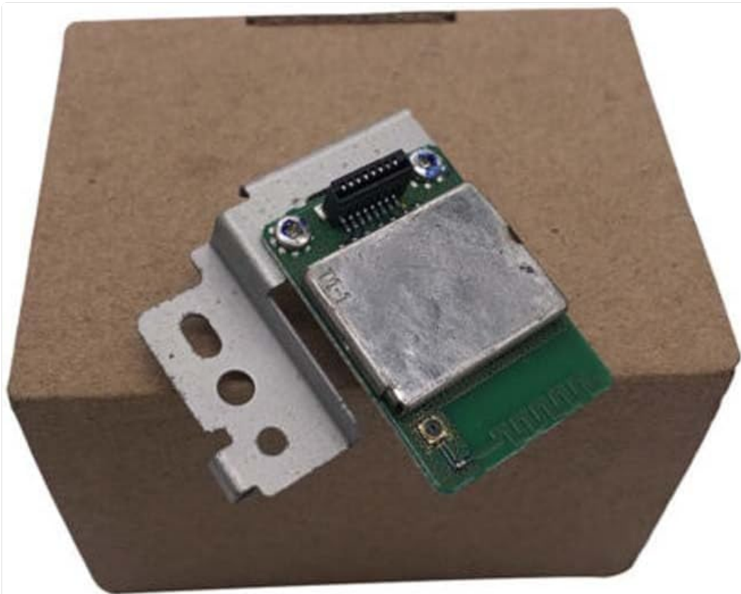
Figure 2: Back view of the CaoDuRen K30357 QM7-3166 WiFi Module. This image displays the underside of the module, featuring a metal shield and the connector pins, also placed on a brown cardboard surface.
