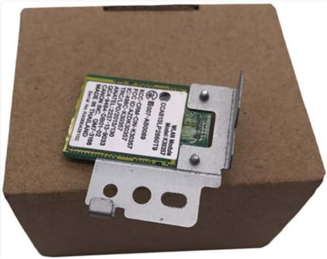
Figure 1: Front view of the CaoDuRen K30357 QM7-3166 WiFi Module. This image shows the module's top side with visible circuit board components and a metal bracket, resting on a brown cardboard surface.
