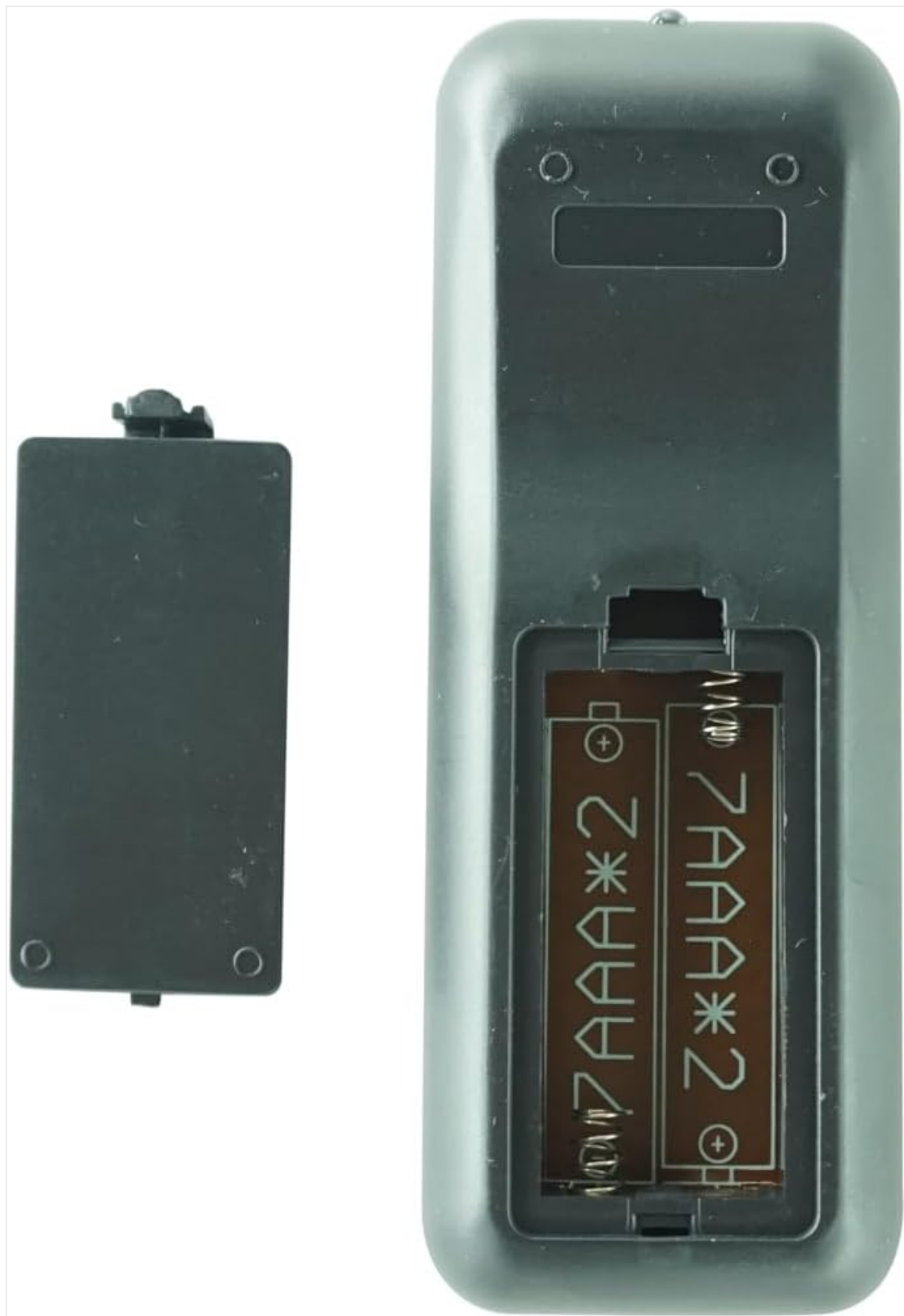
Image: Back of the remote control with the battery cover removed, revealing the two AAA battery slots. The battery polarity markings are visible.
