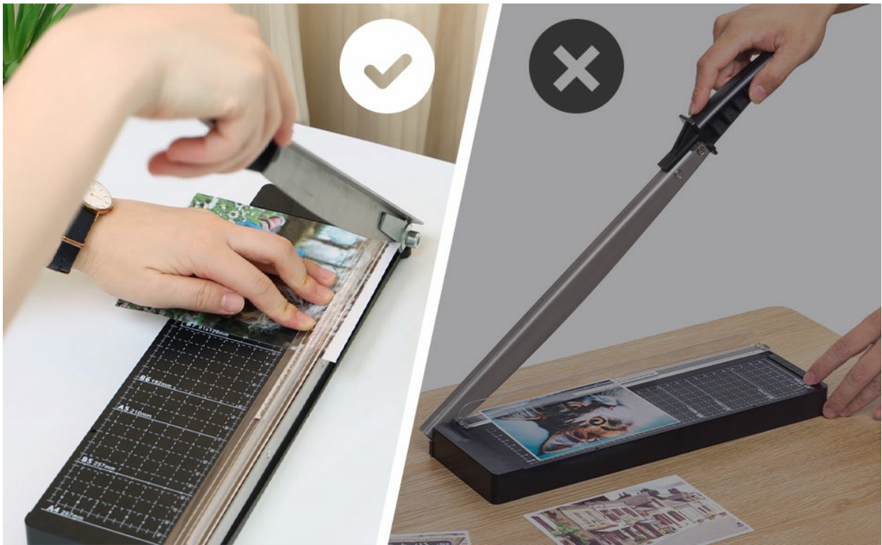
Image: Comparison of correct and incorrect hand placement during cutting, emphasizing safety and proper technique.
