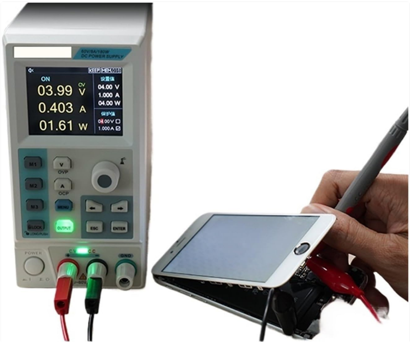
Figure 4.2: The UDP6721 connected to a device, demonstrating a typical application setup.
