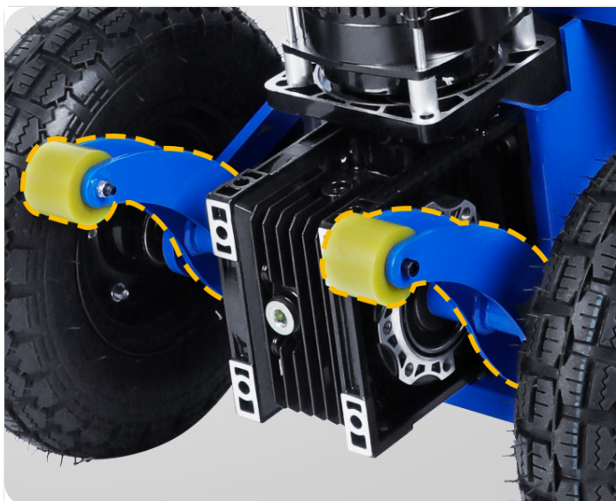
Image 3.3: Detail of the S-shaped support arm.
