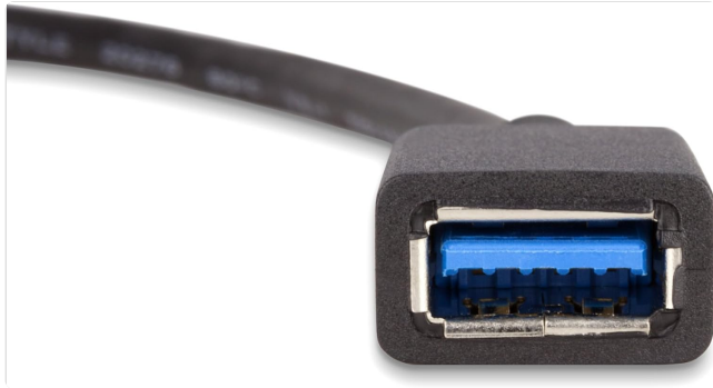
Image: A close-up of the USB-A female port, showing the blue internal tab indicating USB 3.0 compatibility (though product description states USB 2.0 standard).
