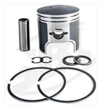
The image above displays the typical contents of the PWC 900 Engine Piston Kit, which includes the main piston unit, a wrist pin for connecting the piston to the connecting rod, and a set of piston rings designed to seal the combustion chamber and control oil. Small circlips are also included to secure the wrist pin.
