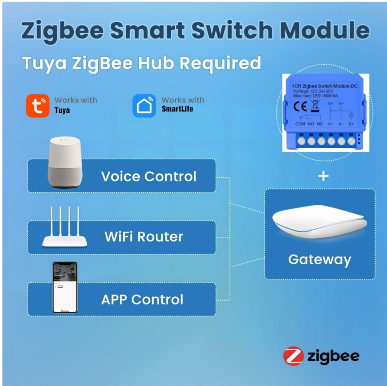
Image 3.2: Diagram illustrating the MHCOZY ZIGDC32 Zigbee Smart Switch Module's integration into a smart home. It shows the module connecting to a Gateway (Zigbee Hub), which then connects to a WiFi Router, enabling APP Control and Voice Control via devices like Google Home. A Tuya Zigbee Hub is required.
