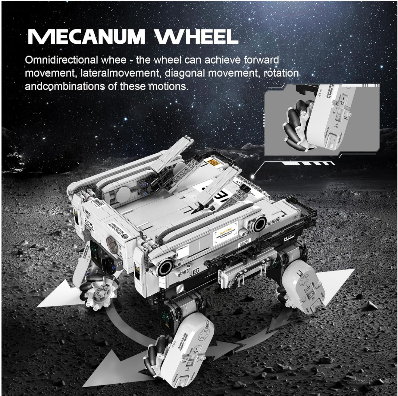
Image: The Mecanum wheels enable versatile movement, including side-slip driving and rotation.
