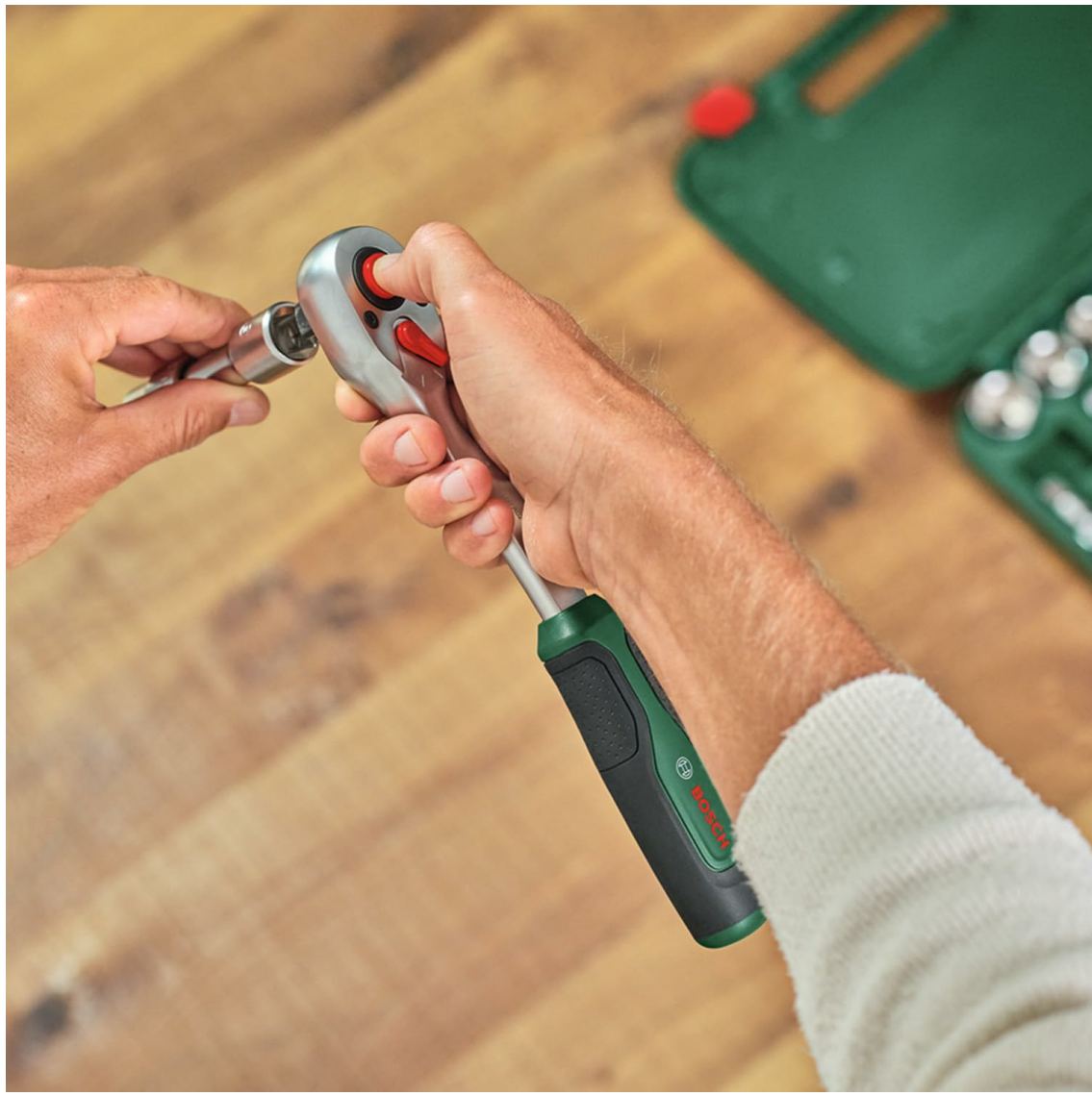
Figure 3.1: Attaching a socket to the ratchet head. Ensure it clicks securely into place.
