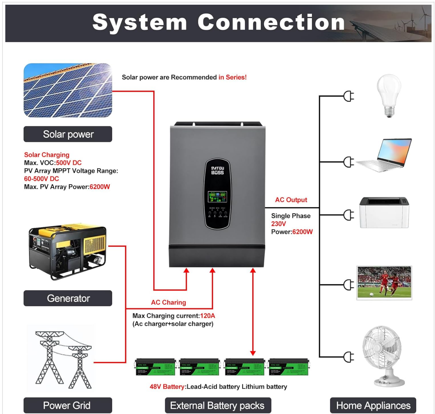
Figure 4.2: Diagram illustrating the system connection of the inverter with solar, battery, grid, and loads.
