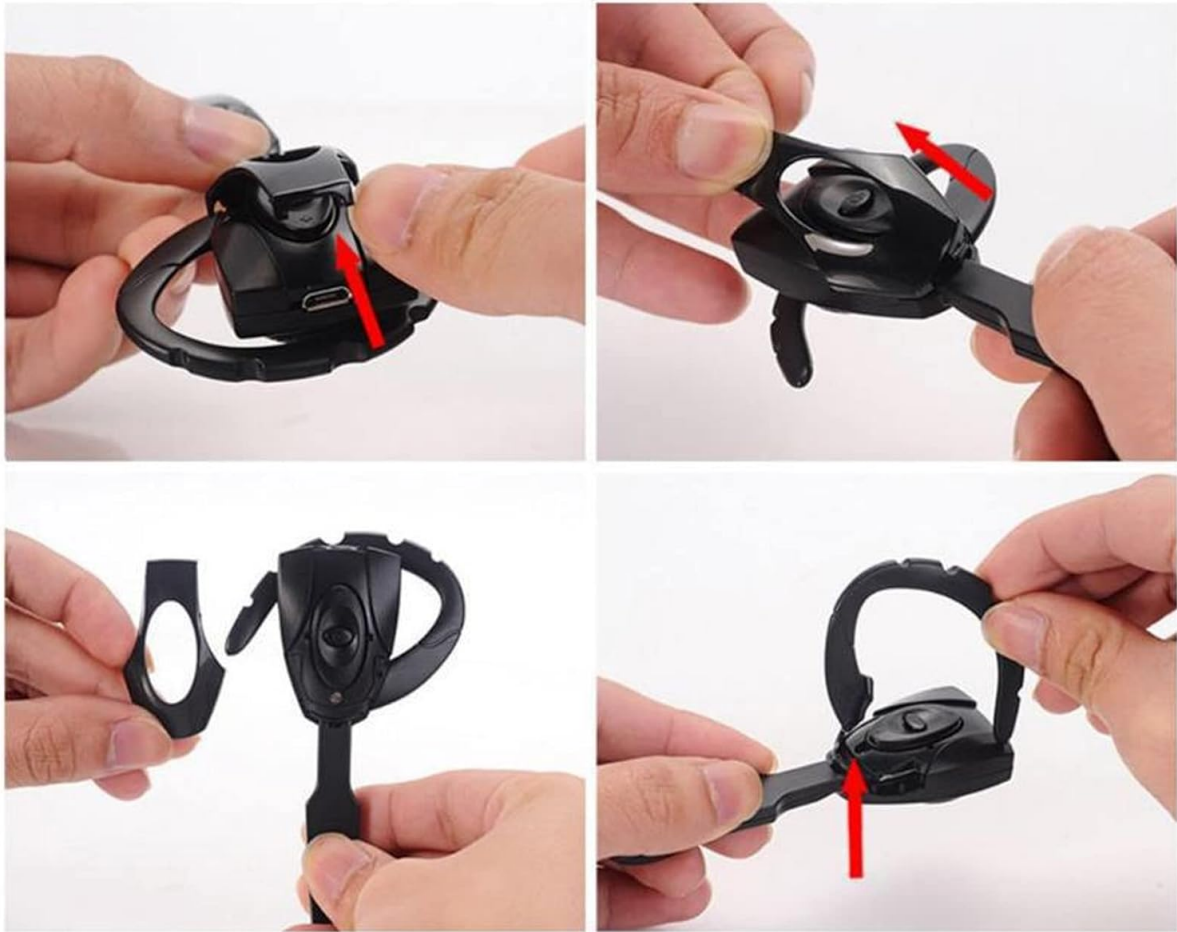
Figure 4.2: Ear Hook Installation and Charging Port Access. This series of images illustrates the steps for attaching and removing the ear hook, as well as locating the charging port on the earpiece.
