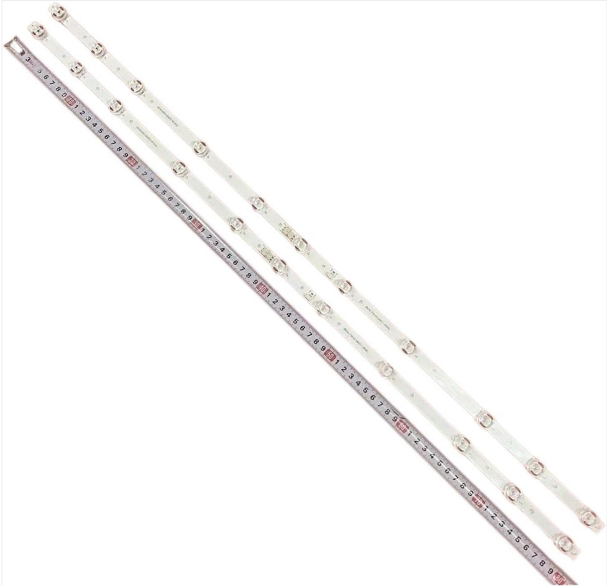
Figure 1: Overview of two LED backlight strips. A measuring tape is placed alongside them, indicating a length of approximately 80.5 cm (805 mm) for each strip. This image helps in verifying the physical dimensions of the replacement parts.
