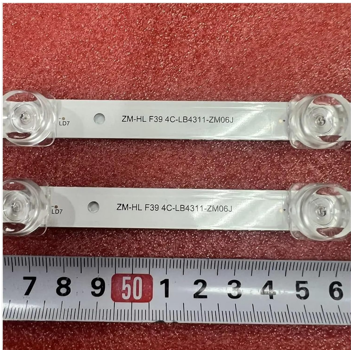
Figure 3: Close-up of the LED strip displaying identification markings such as "ZM-HL F39 4C-LB4311-ZM06J". These markings are crucial for confirming compatibility with the original TV backlight strips. A ruler is visible at the bottom for scale.
