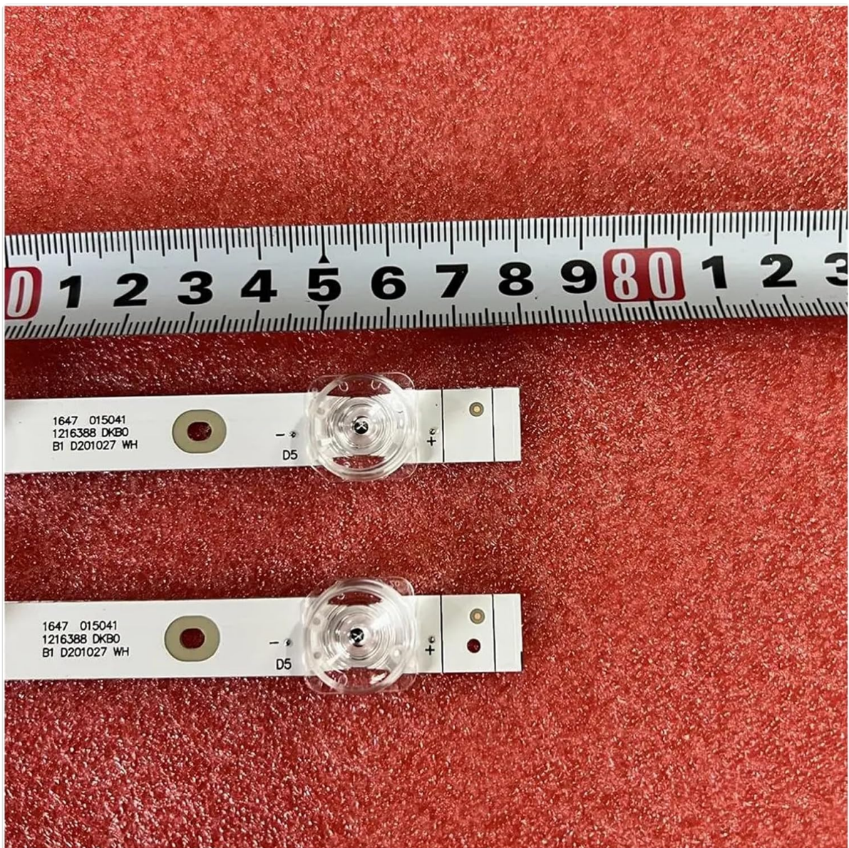
Image 4.3: End section of an LED backlight strip. This image focuses on the connection points and the arrangement of LEDs at the strip's extremity, providing a clear view of how the strips connect to the TV's power board or to each other.
