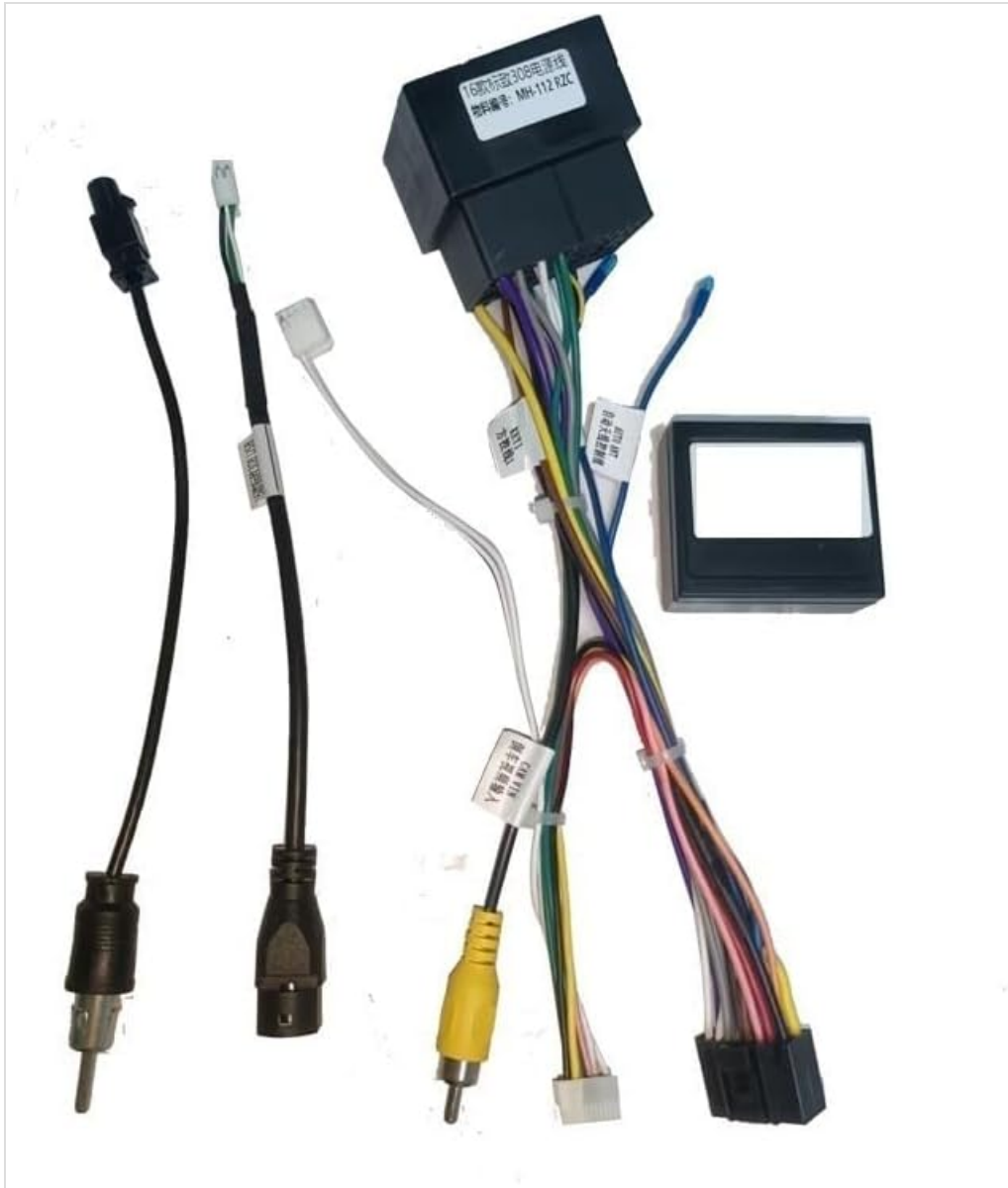
Figure 1: Overview of the YTRIO 16-pin wiring harness and Canbus box. This image displays the main wiring harness with its various connectors, including the 16-pin main connector, RCA cables, antenna adapters, and the Canbus box module.
