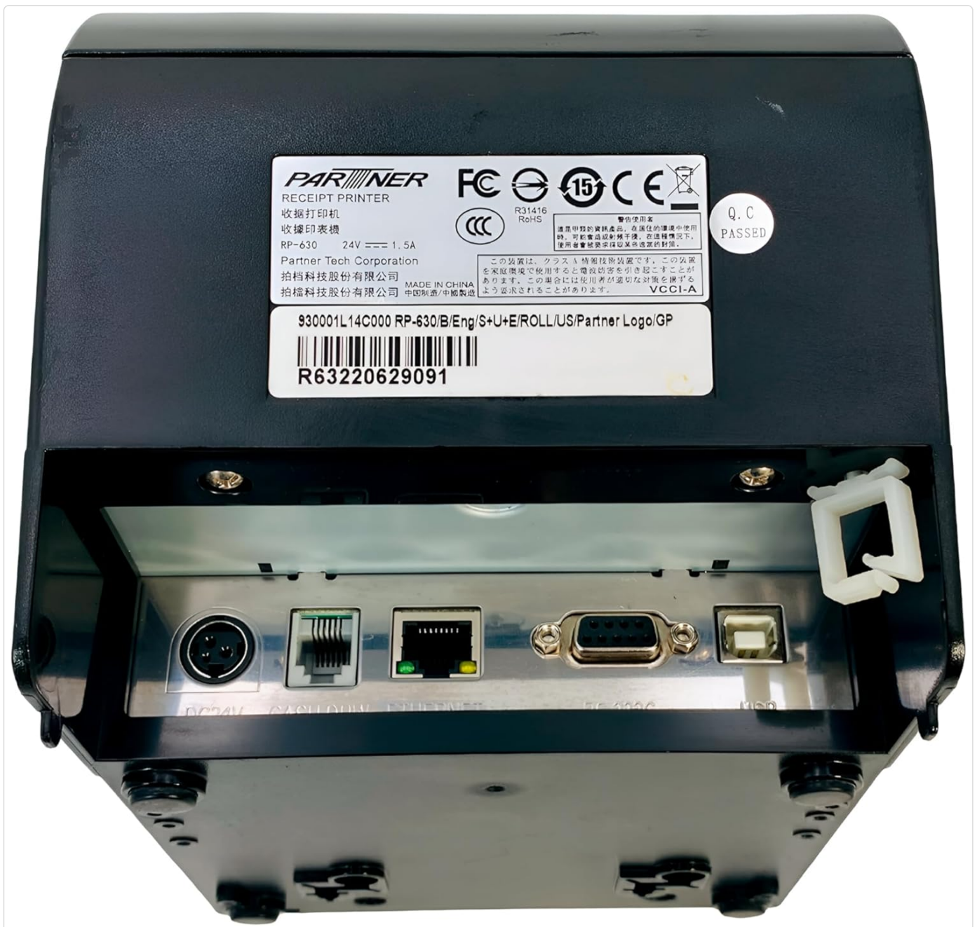
Figure 2: Rear view of the RP-630 printer, highlighting the USB, Serial, and LAN (Ethernet) connectivity ports. The label on the back indicates serial number R63220629091.
