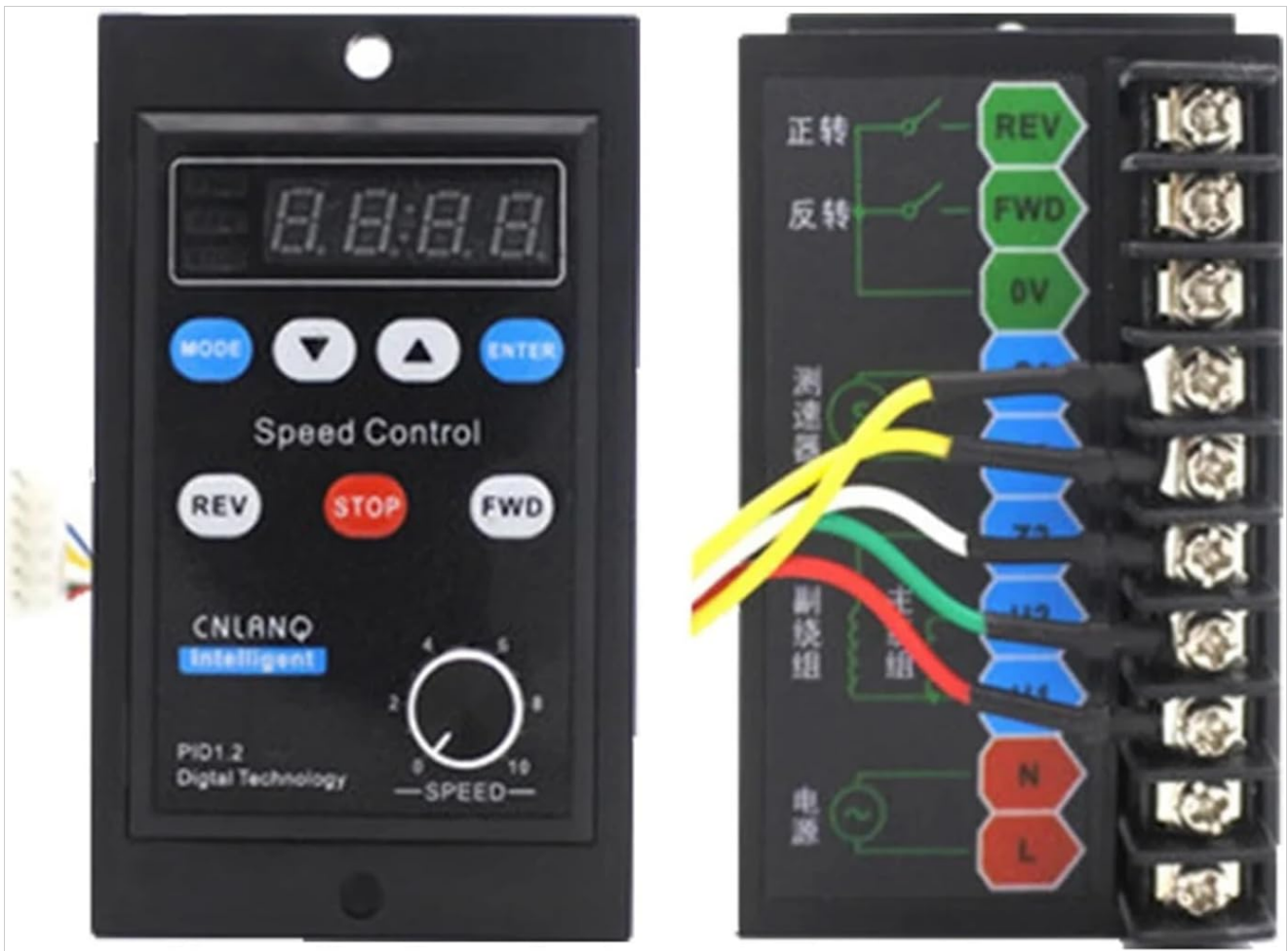
Figure 4.1: Detailed view of the rear terminal block. Connections include: REV (Reverse signal), FWD (Forward signal), 0V (Common ground), Speed Feedback (yellow, white, green wires), N (Neutral AC 220V), L (Live AC 220V).
