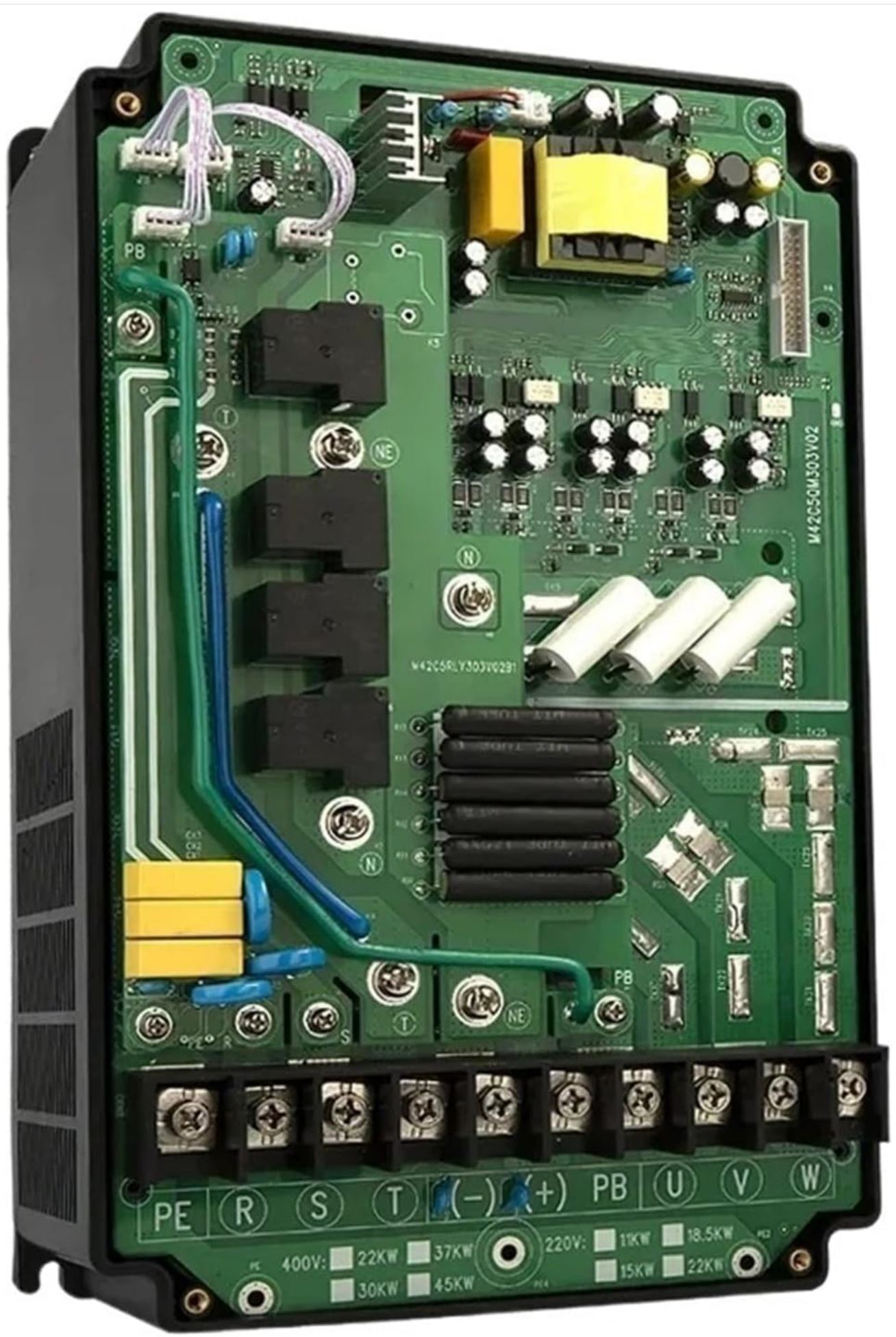
Figure 5.1: Internal view of the VFD showing the terminal block layout for power and control connections.
