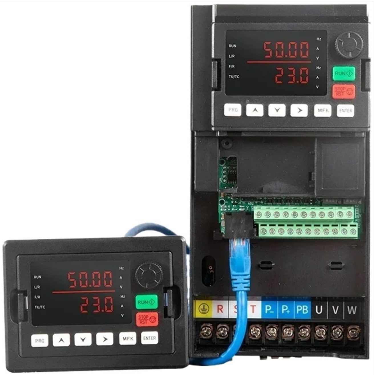
Figure 3.2: The SU800 VFD connected to an external control panel, demonstrating remote operation capability.
