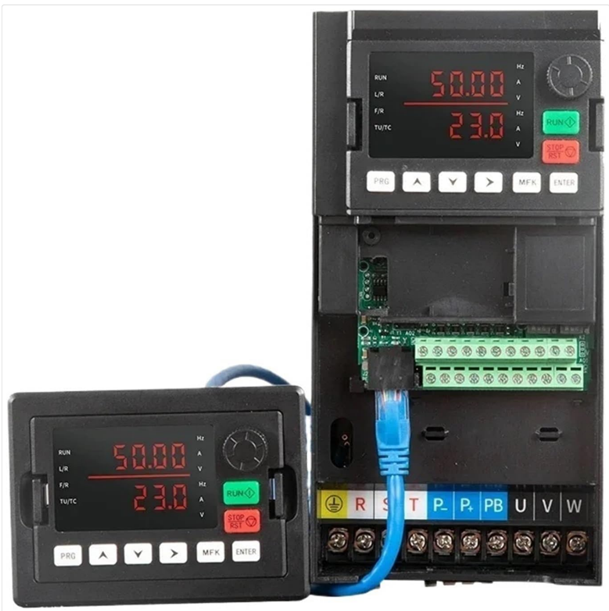
Figure 5.1: VFD showing the main unit, remote control panel connection, and clearly labeled power and control terminals (R, S, T for input; U, V, W for motor output; PB for braking resistor; PE for ground).
