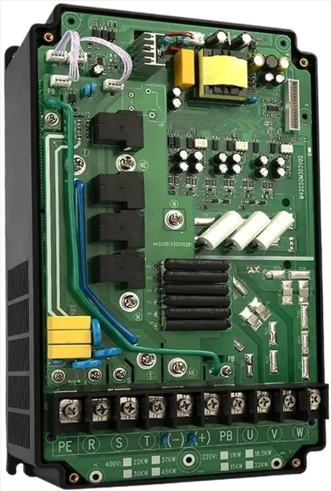
Figure 3.2: Internal view of the VFD's circuit board, illustrating component layout and robust design.
