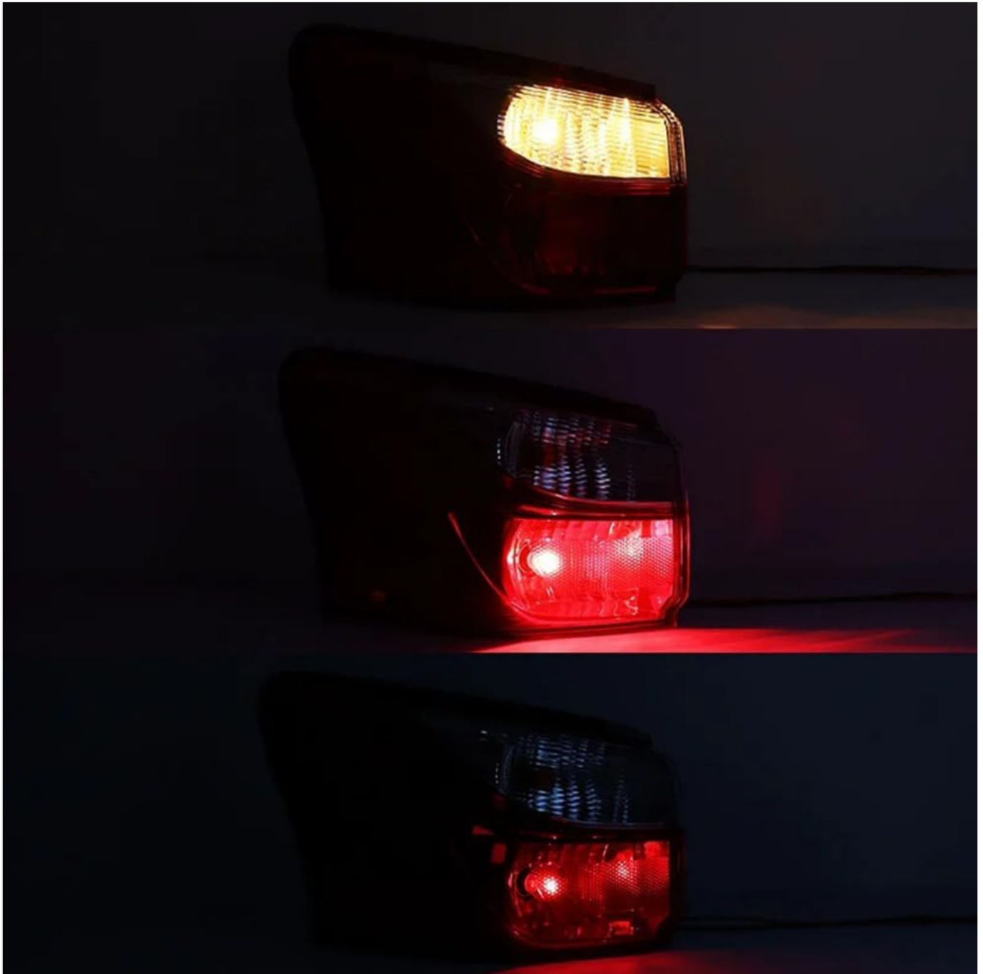
Figure 5.1: Examples of the tail light assembly in operation, demonstrating turn signal, brake, and running light functions.
