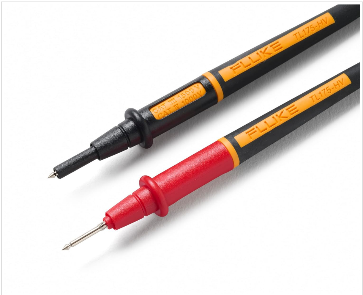
Figure 3: Test leads with TwistGuard tips retracted for CAT II measurements (19mm exposed tip).
