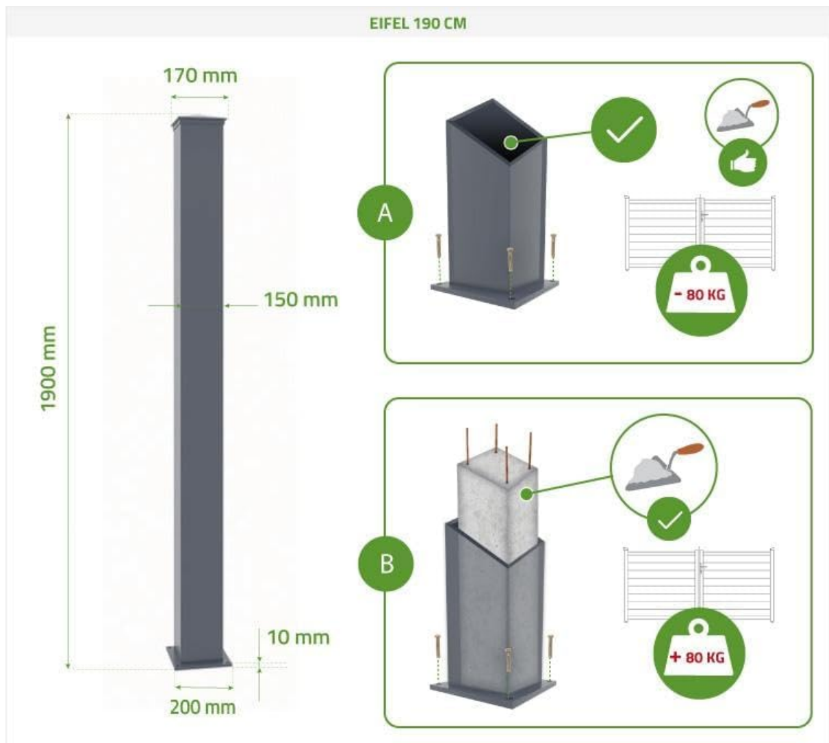
Figure 4.1: Post installation methods for the EIFEL 190cm posts. Method A shows surface mounting with bolts, while Method B illustrates embedding the post into a concrete foundation, emphasizing the need for at least 80kg of concrete for secure installation.
