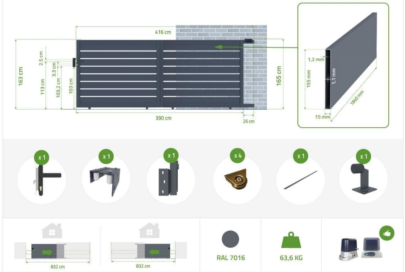
Figure 3.1: Overview of the VOGEL 400C160 gate with dimensions and main components. This image illustrates the gate's overall size, including its 390 cm width and 163 cm height, along with a visual representation of the various parts included in the package, such as the gate panels, posts, and hardware.
