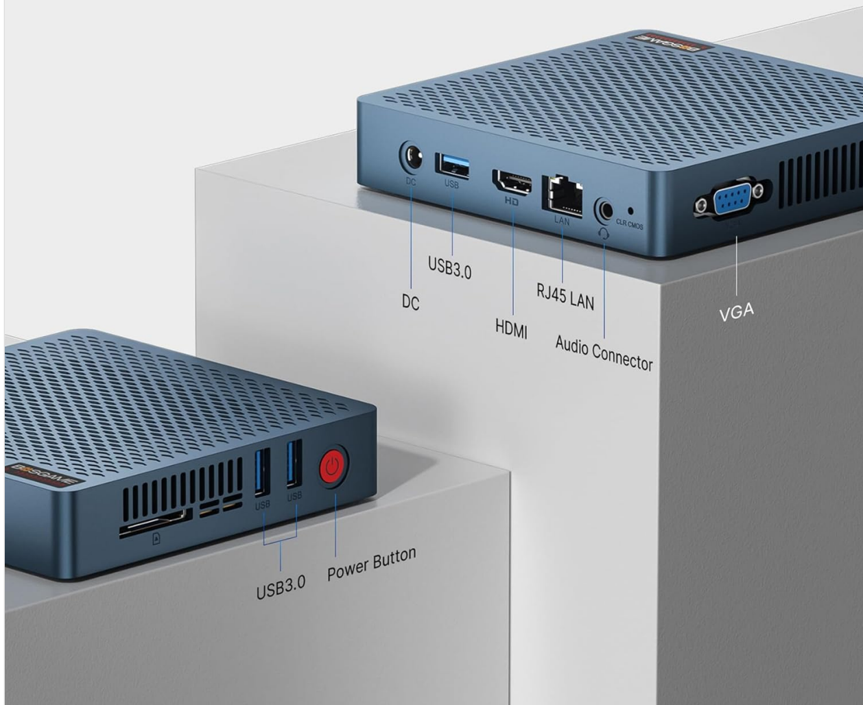
Figure 2.3.2: Detailed view of the BOSGAME AG40 Mini PC ports and power button.
