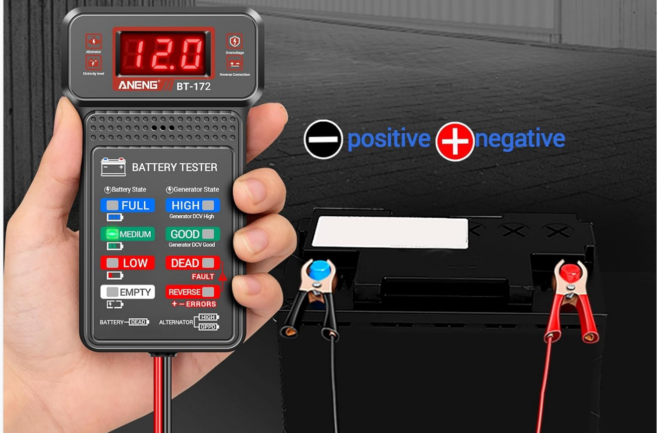
Figure 4.6: Proper connection of positive and negative alligator clips to the battery terminals.
