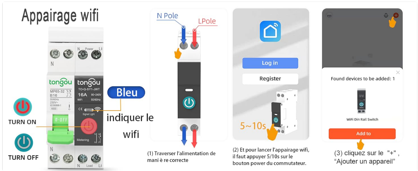
Figure 6: Step-by-step guide for pairing the device with the Tuya/Smart Life app, showing the blue Wi-Fi indicator and app interface.
