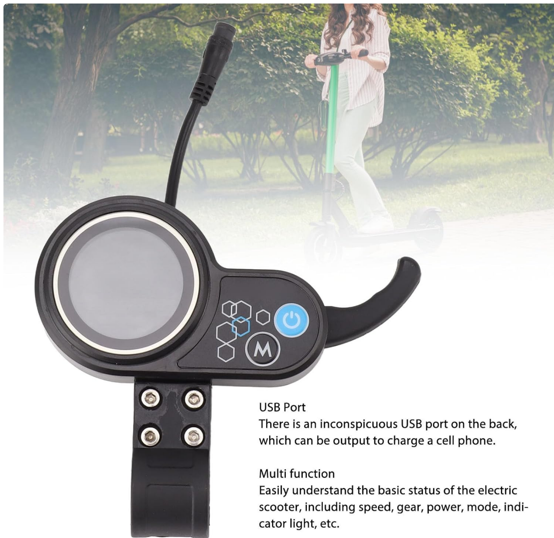
Figure 5: The display panel, illustrating the location of the USB charging port on the back.
