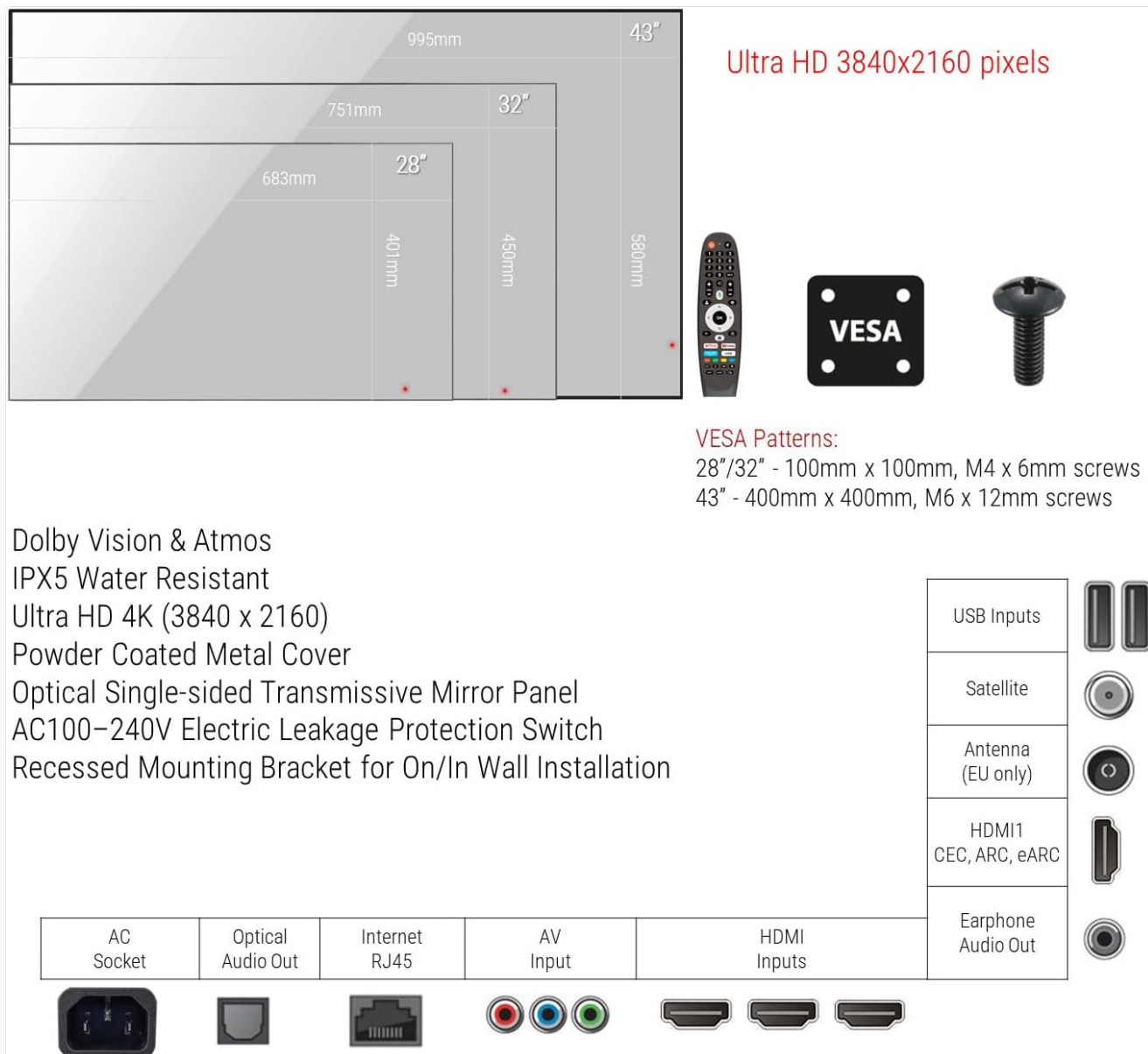
Figure 5.1: VESA mounting patterns and port overview.
