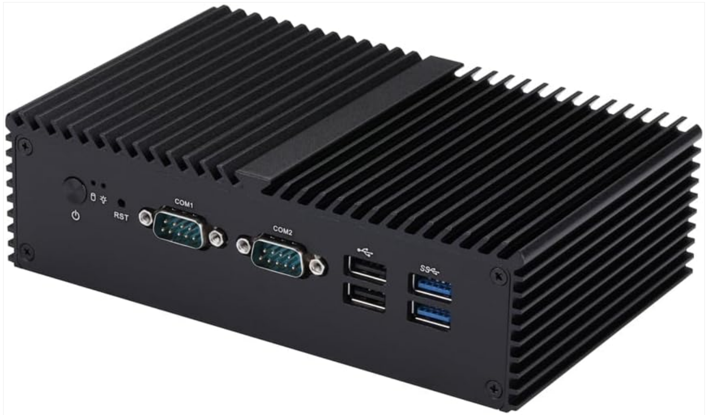
Image: Front view of the Qotom Q790X Mini PC, displaying the power button, reset button, and two COM ports (COM1, COM2).
