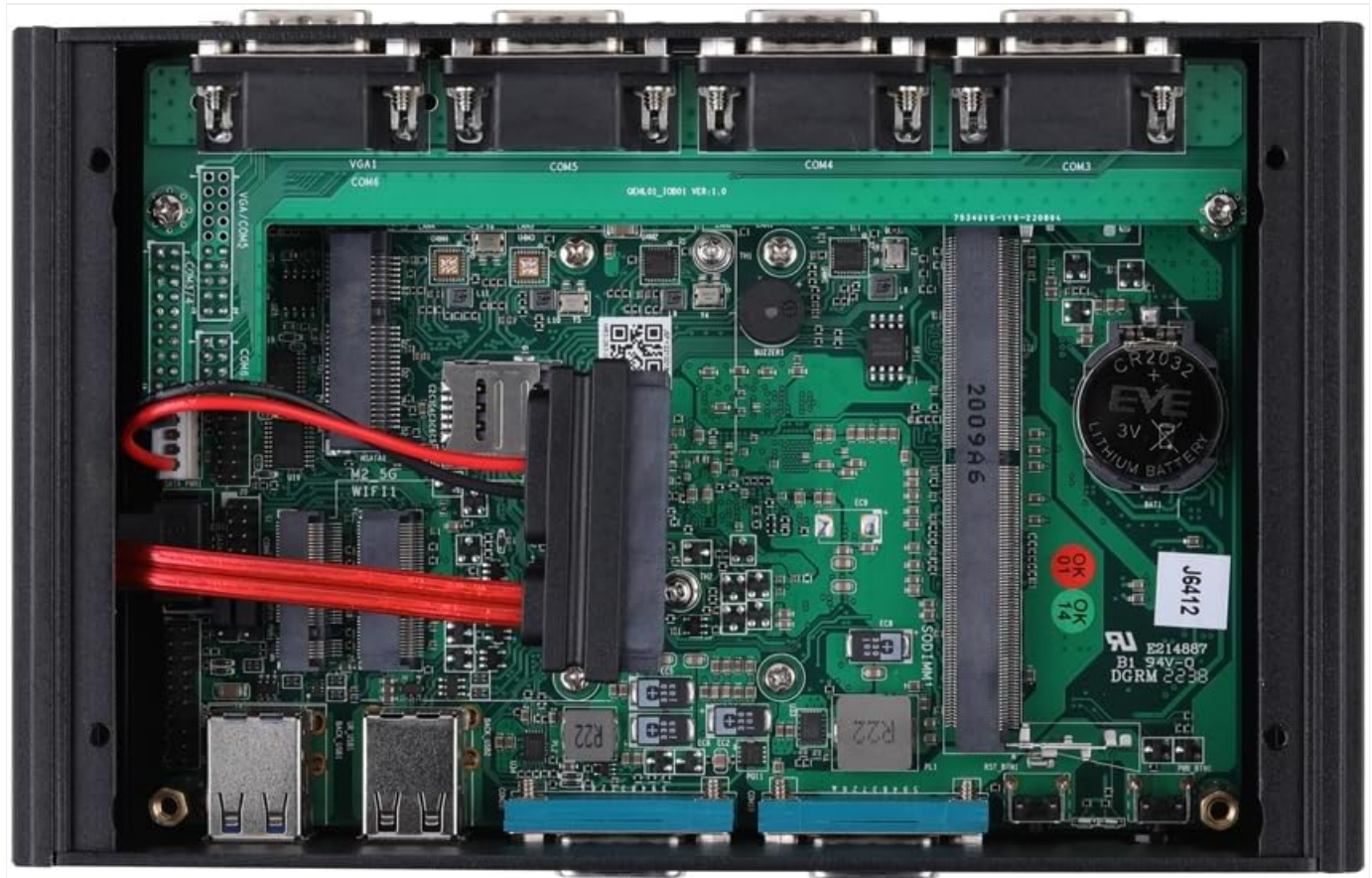
Image: Internal view of the Qotom Q790X motherboard, highlighting the DDR4 SO-DIMM RAM slot, mSATA SSD slot, and a 2.5-inch SATA data/power connector for additional storage.
