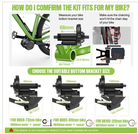
This image illustrates how to accurately measure your bike's bottom bracket shell width and internal diameter using calipers or a ruler to confirm compatibility with the BAFANG mid-drive motor. Ensure the chainring will not interfere with the chain stay.
