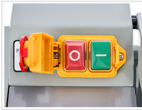
Image: Close-up of the power and emergency stop buttons for quick machine control.
