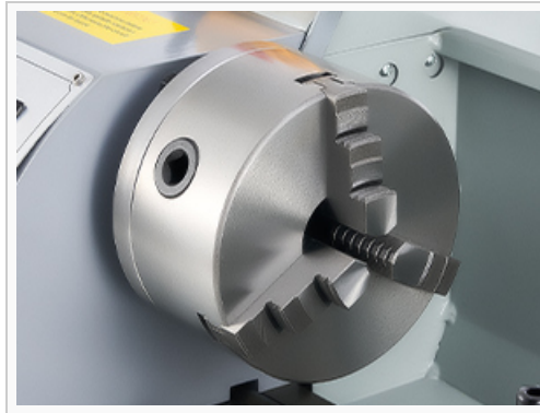
Image: Close-up of the 3-jaw chuck, used for holding workpieces.
