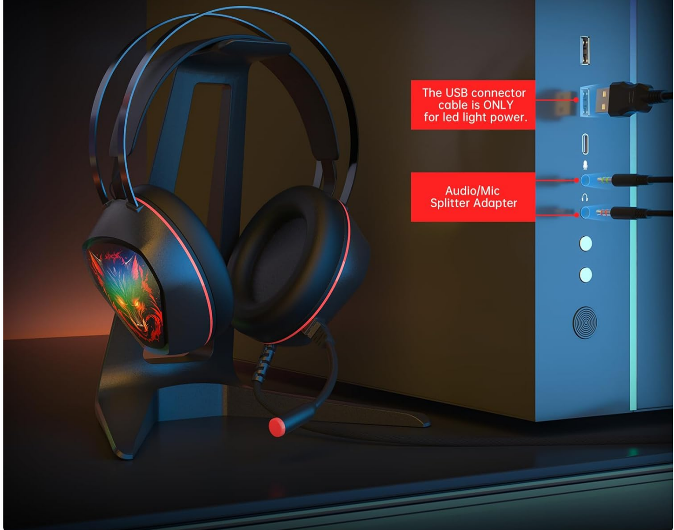
Figure 3.1: PC Connection with USB for RGB and Audio/Mic Splitter
