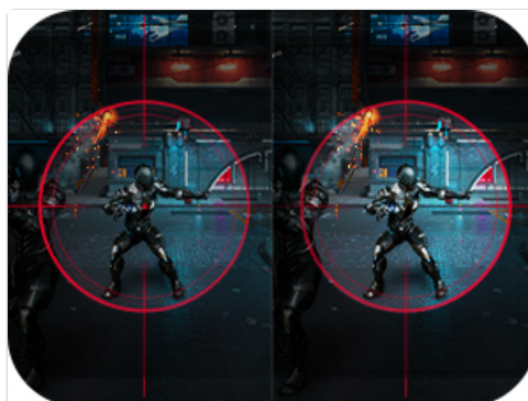
Figure 3.6: Comparison showing the effect of Black Stabilizer, making dark in-game areas more visible without overexposing bright areas.
