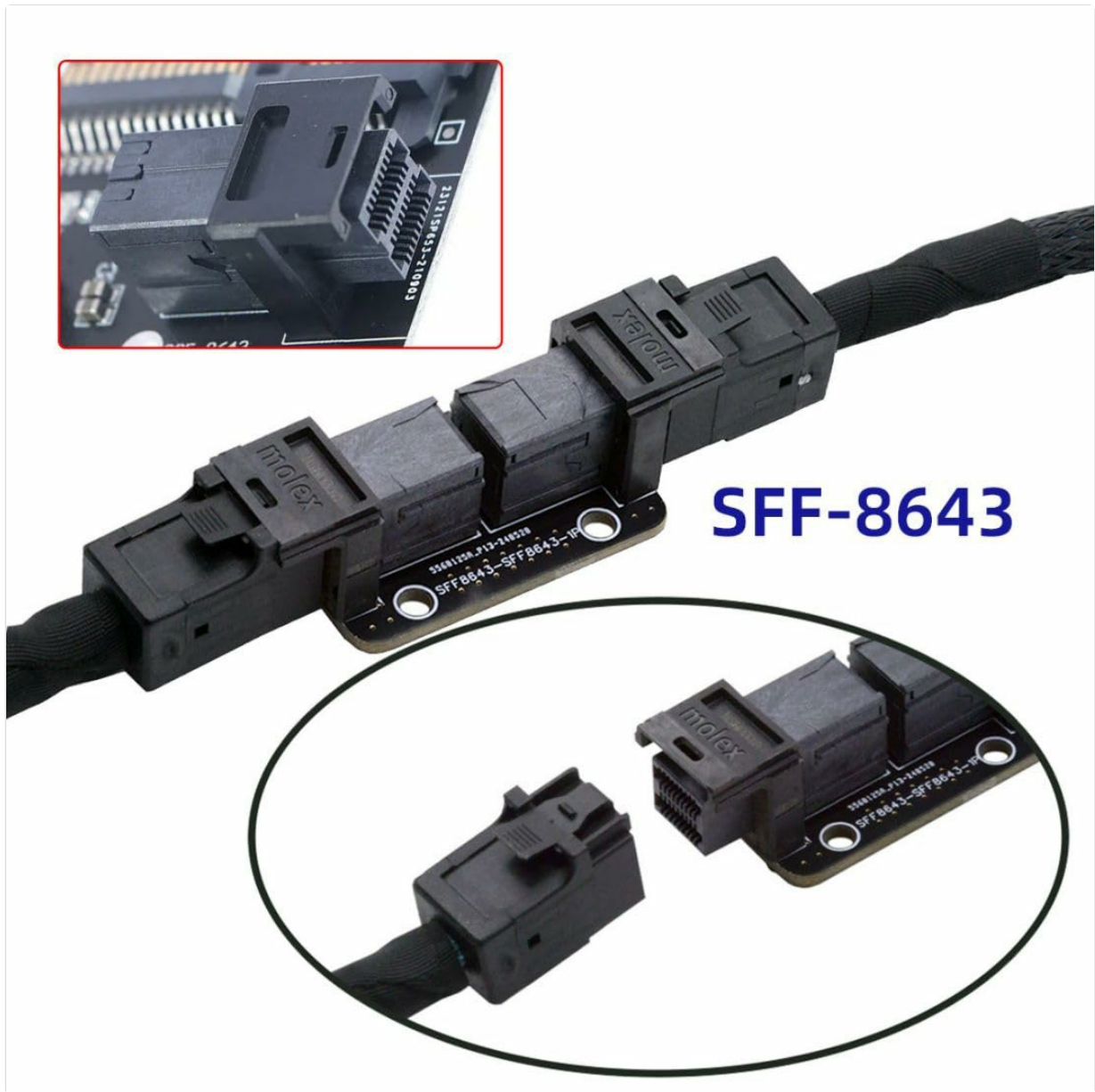
Image 3.2: An example of an SFF-8643 cable connected to the adapter. This image shows the adapter in line with a cable, demonstrating how the female-to-female connection is established to extend or join two SFF-8643 cables.
