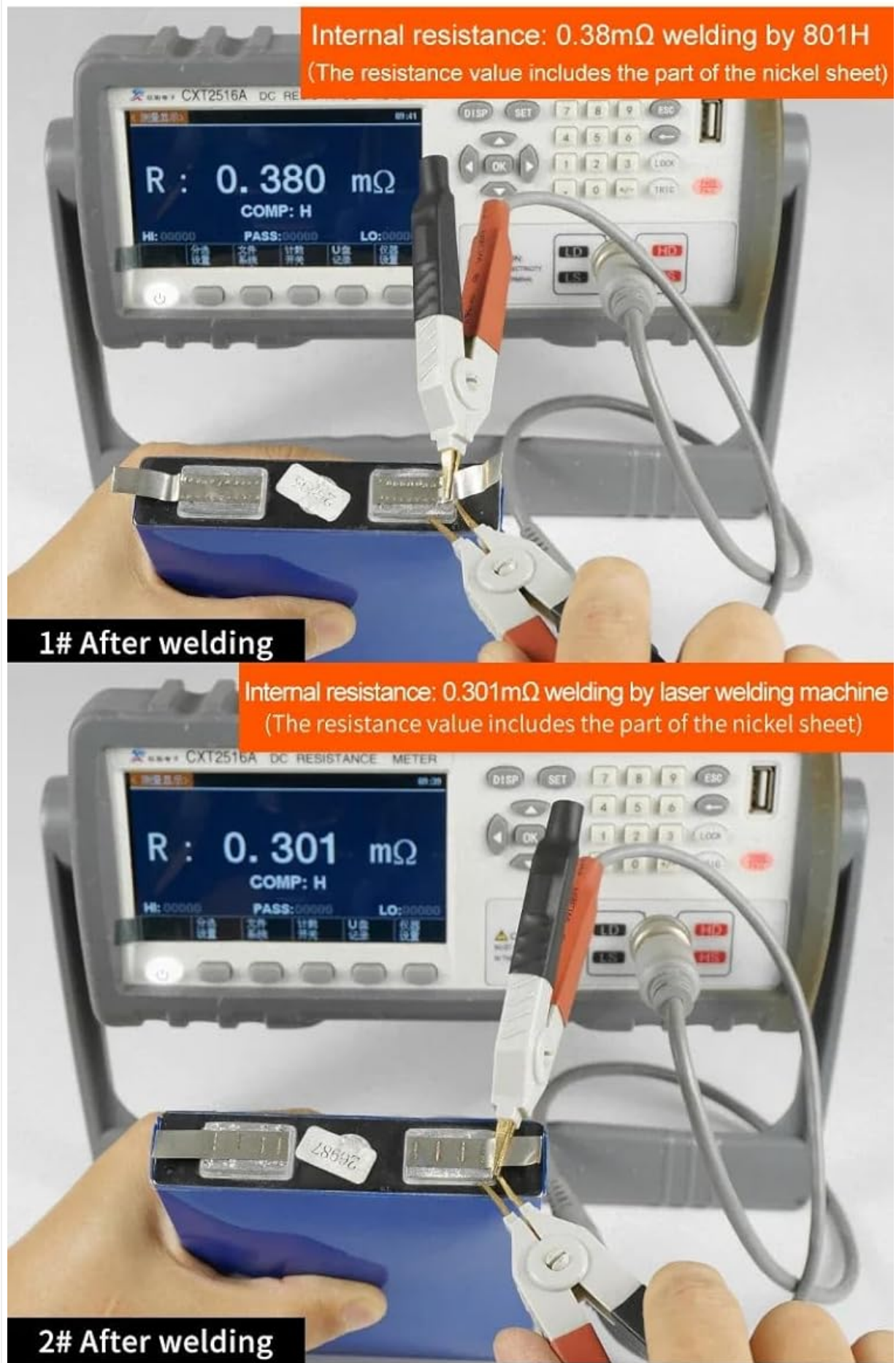
Figure 8.1: Example of a solder joint effect performance test, measuring internal resistance to assess weld quality.
