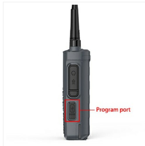
Figure 7.1: Program Port. This image shows the location of the program port on the side of the radio, which may be used for manual software updates or advanced configuration.
