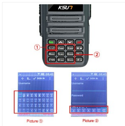
Figure 5.6: Numeric Keyboard Mode. This image shows the radio's display in numeric input mode, useful for entering numbers or special characters.
