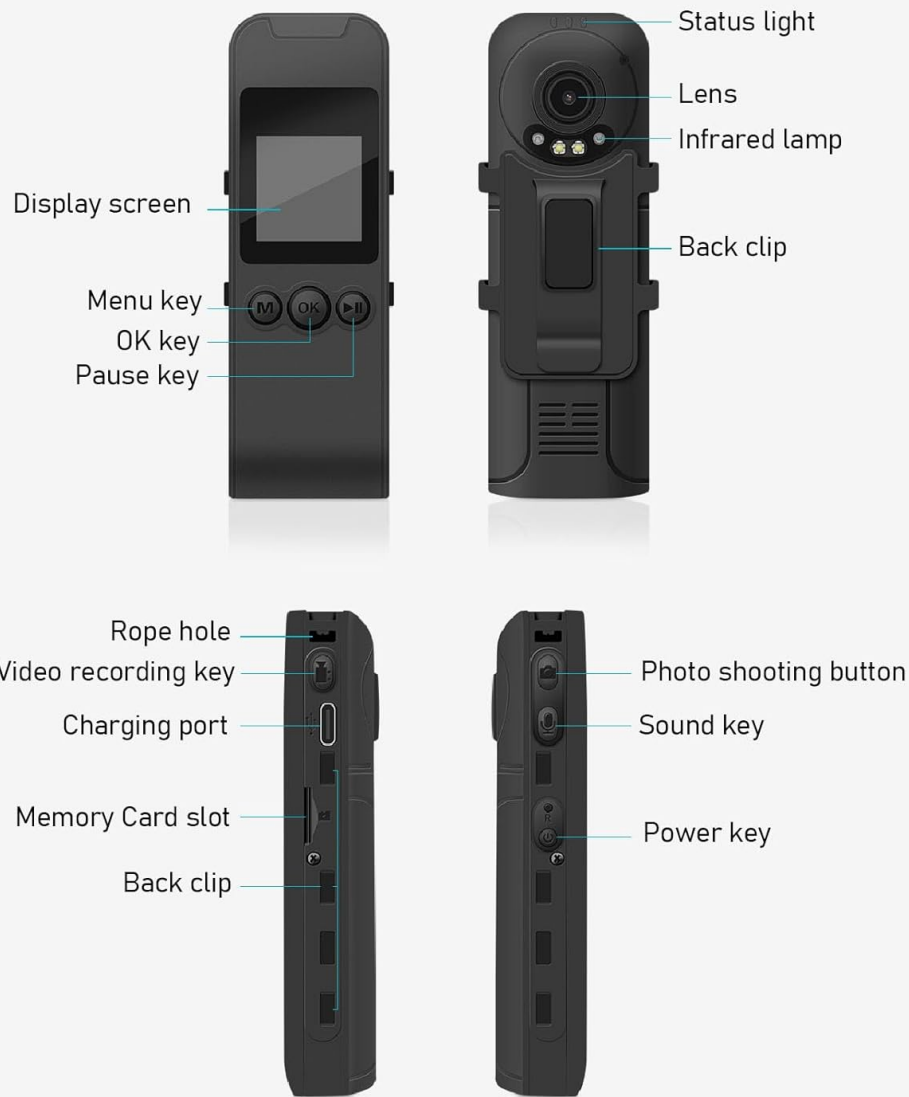
Figure 3: Labeled components of the Cuifati Mini Body Camera.
