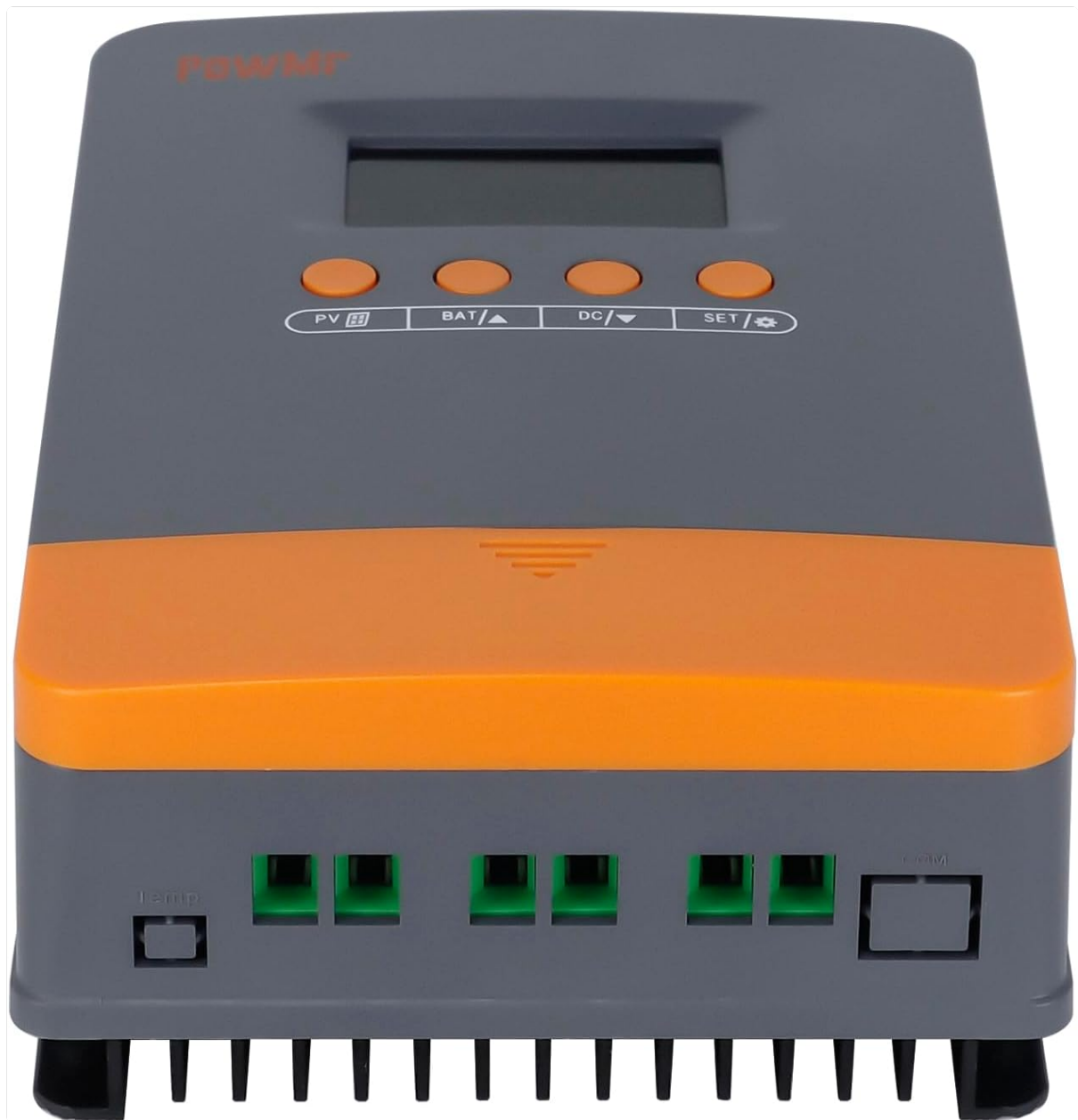
Figure 1: Front view of the PowMr 45A 100V MPPT Solar Charge Controller. It features an LCD display and control buttons for easy operation. The bottom section includes terminals for solar panel, battery, and load connections, along with a temperature sensor port and a communication port.
