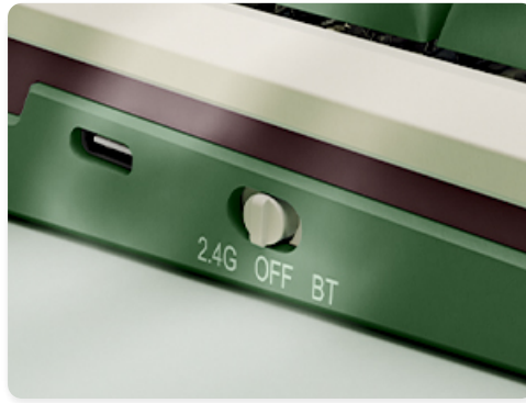
Image: Detailed view of the USB-C port and the 2.4G/OFF/BT switch on the keyboard's side.
