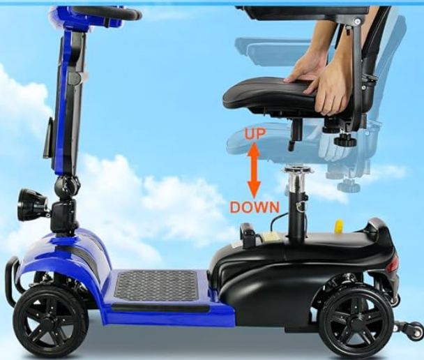
Step 1: Remove the seat
