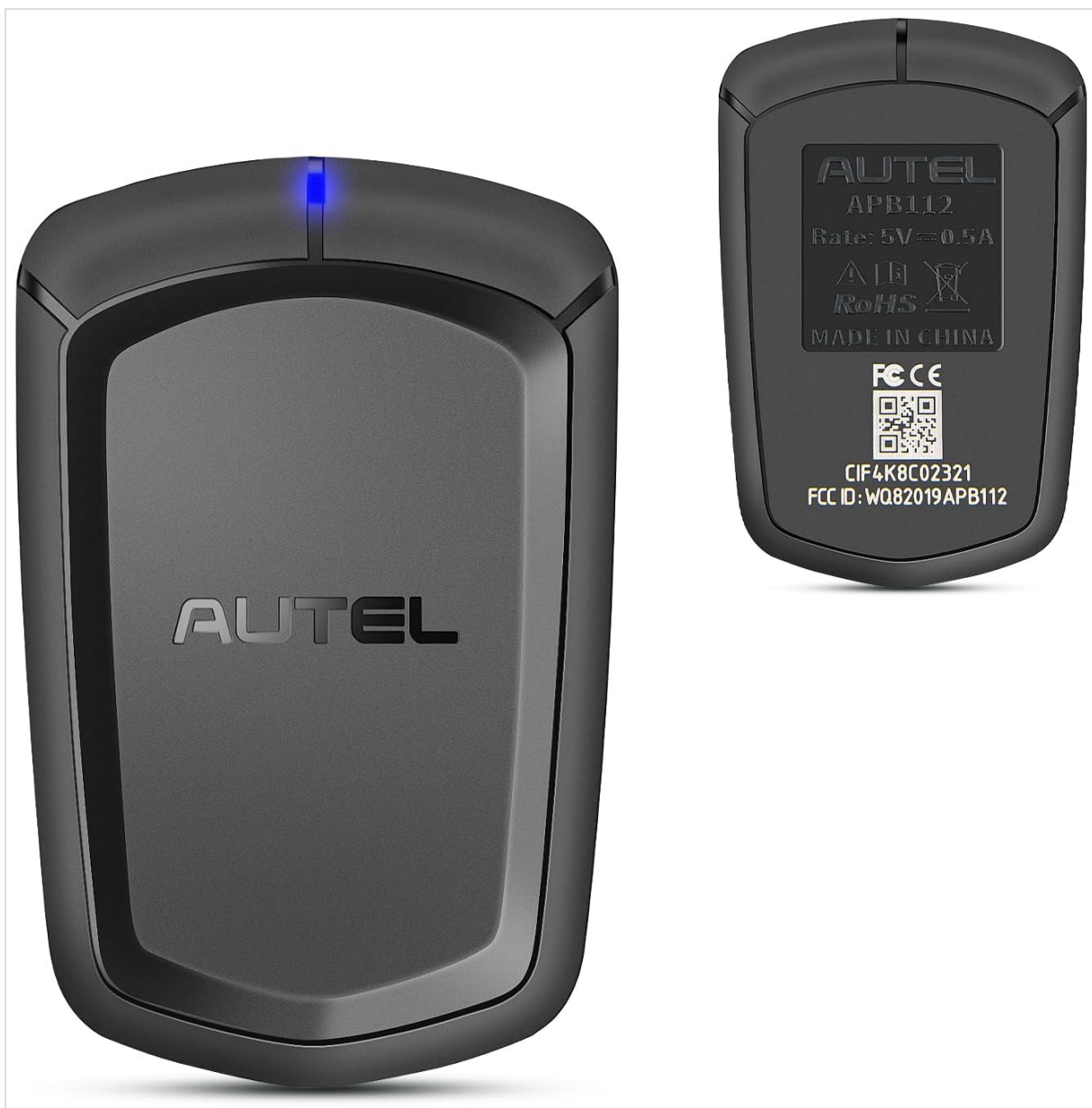
Figure 4.2: Back view of the APB112 device, displaying the model number (APB112), power rating (5V=0.5A), RoHS compliance, FCC ID (WQB2019APB112), and manufacturing origin.
