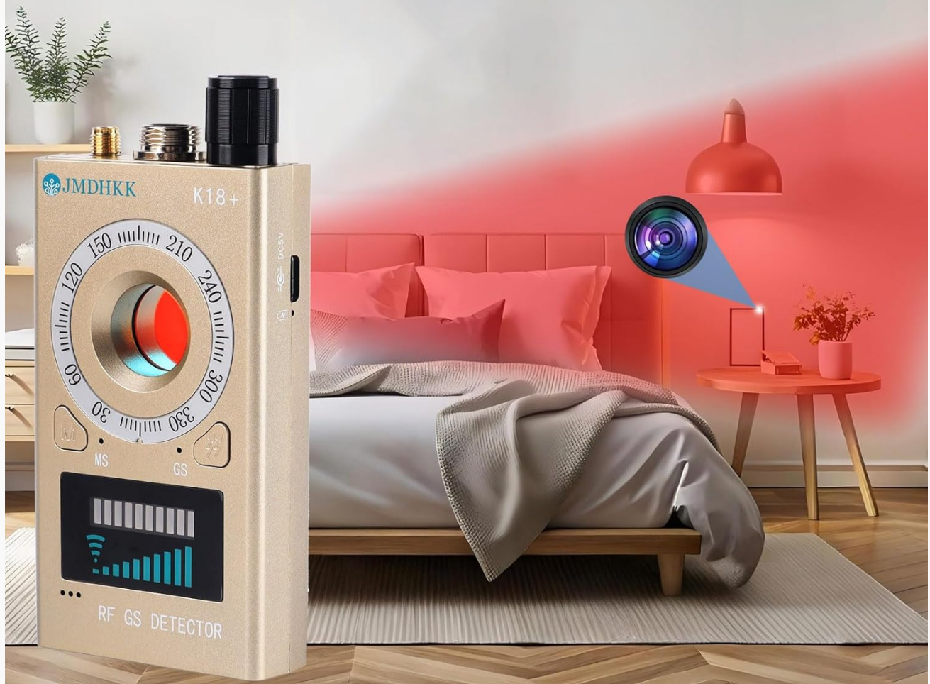
Image 3: Using the K18+ for hidden camera detection. The red light emitted by the device helps reveal reflective camera lenses.
