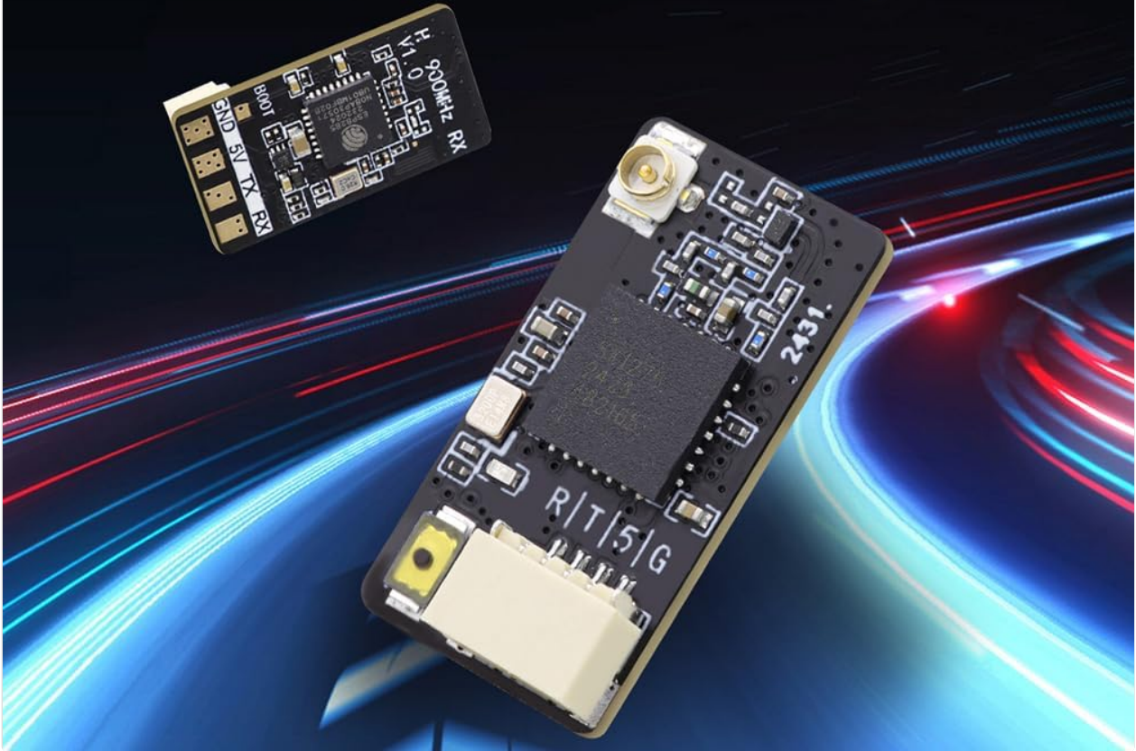
Image: The HGLRC ELRS 915MHz Nano Receiver with its T-type antenna connected, highlighting its long-range communication capability.
