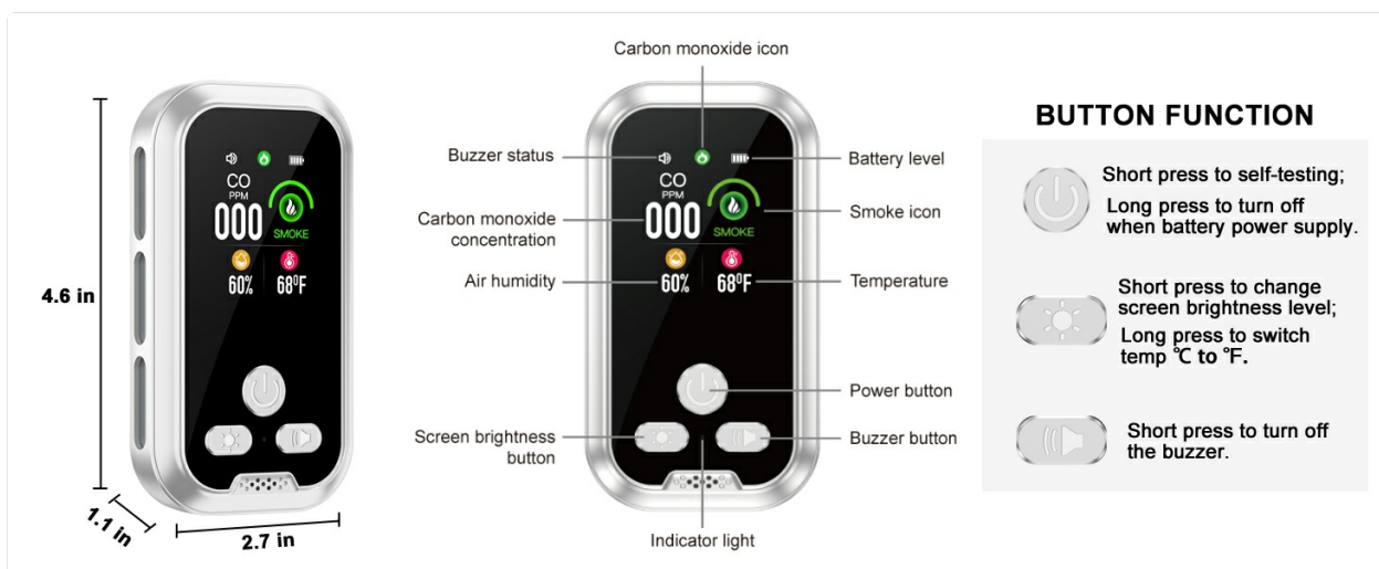
Image 3.3: Detector screen elements and button functions.
