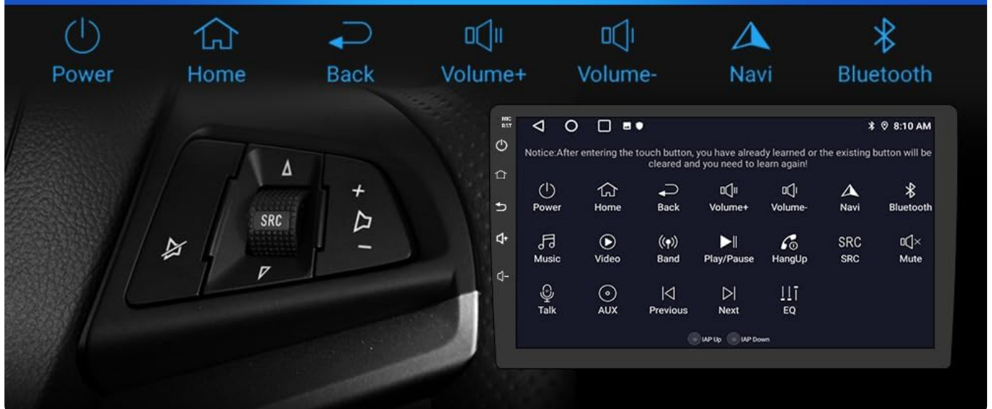
Figure 4.11: Steering wheel control integration.
