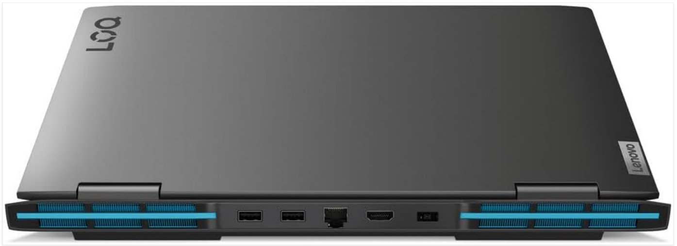
Figure 3: Rear view of the laptop, highlighting the power input and other ports.
